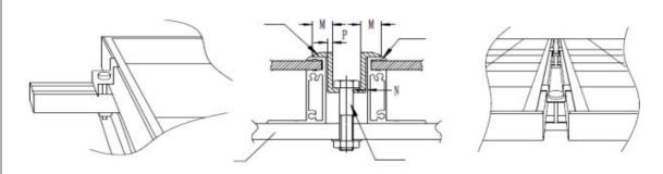
Dimension "M" represents the mounting overlap dimensions for clamp and moudule frame fronts;
